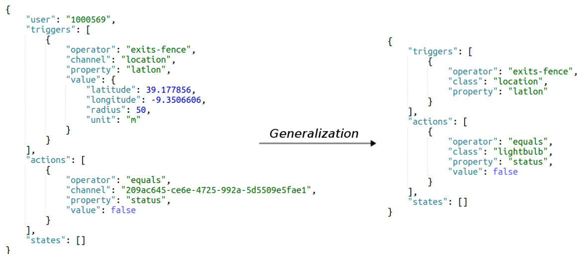
Figure 4.1: Generalizing from an automation instance to a template. Channel is the device identifier.
